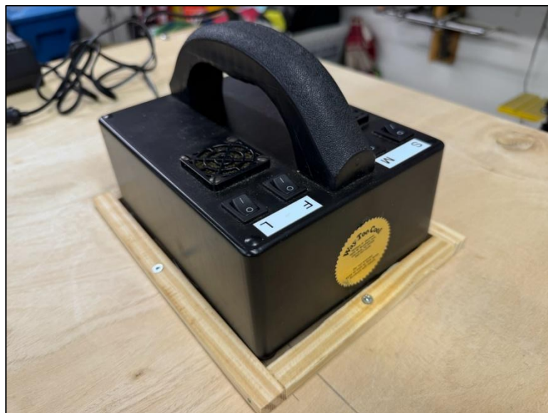
Figure 3 —UV showcase under assembly, with a donated three-tube Way-Too-Cool fluorescent light as the starting point. The light allows fluorescence under shortwave, medium-wave, and longwave ultraviolet light.
