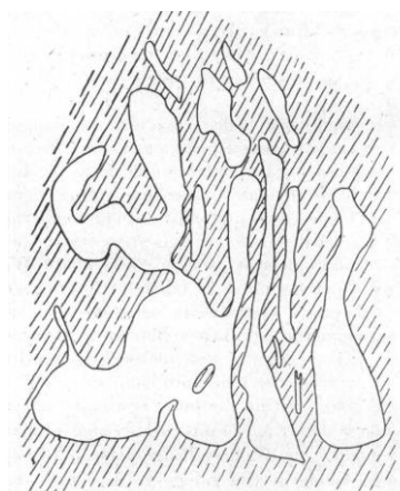
Figure 4 —Sketch of irregular gold-bearing quartz bodies (white) in the Piedmont bedrock (schist, dashed area) at the Laird Prospect in Orange County, to the west of Fredericksburg, VA. Source: Pardee and Park (1942).
