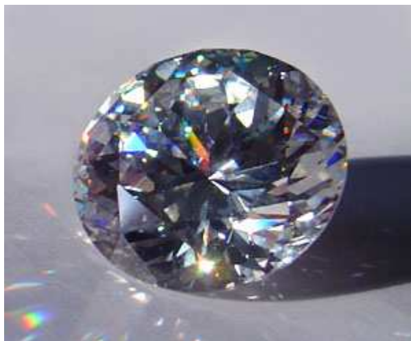
Cubic zirconia (zirconium oxide), a synthetic diamond substitute. Source: Wikipedia.
