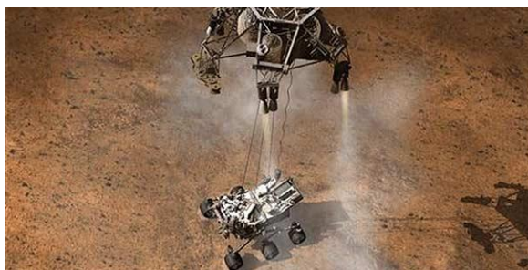
Rocket-propelled crane lowering Curiosity to the surface of Mars.
